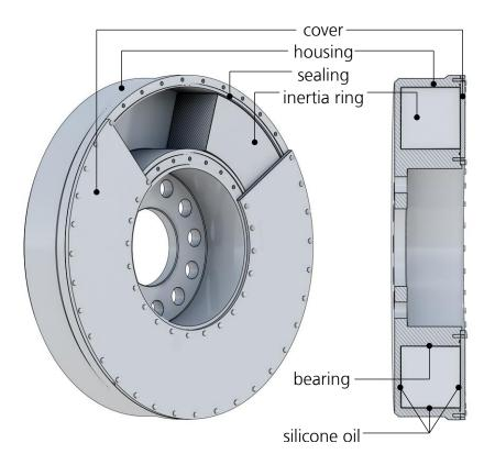
The housing is mounted rigidly to the free end of the crankshaft.
