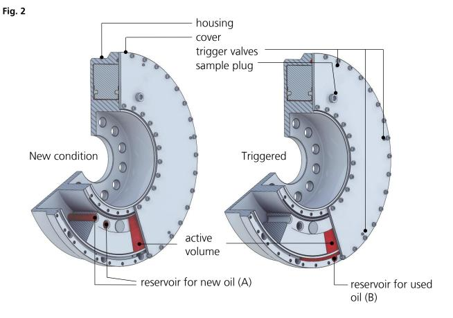
By integrating an additional inner reservoir with new oil (A) into the inertia ring, the damper contains from twice the usual amount of silicone oil. During operation, only the oil in the shear gap is loaded and thus subject to wear, while the oil in the inner reservoir (A) remains unloaded and therefore in new condition.
